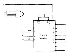
Specify the output line that goes low if the input (Including the enable lines) to the 3x8 decoder (to be used in interfacing a memory chip with 8085) is
